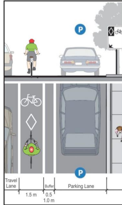
Figure 33: On-Street Bike Lane Cross-Section
