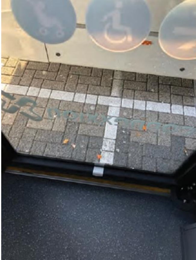
Figure 14 - Example of Alignment Markers Inside/Outside The Bus To Help Operators With Positioning
