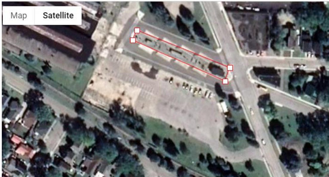
Figure 20 - Enclosed Area Shows the Additional Coverage Of Solar Panels For The Site System Capacity: 163.4 kWdc (1090 m 2 )
