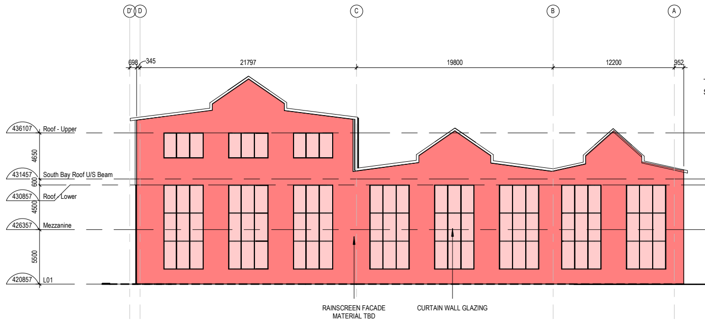
EAST ELEVATION OF NEW FACADE ENVELOPE SCALE = 1:250
